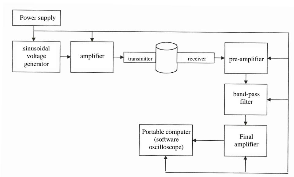
Fig. 3. Block diagram of the rot flaw detector
