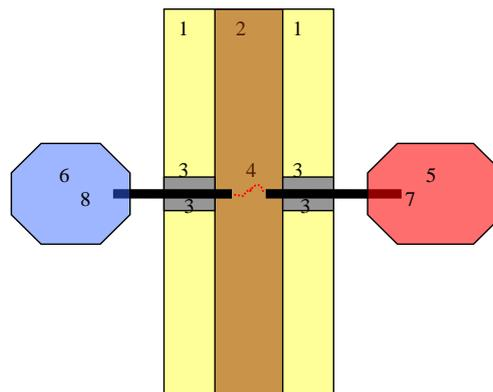
Fig. 12. Idea of the experiment: 1 - sound wood, 2 - destructive rot, 3 - vibration separator, 4 - vibration in the rot, 5 - mechanical frequency generator, 6 - analogue frequency analyser, 7 - transmitting rod, 8 - receiving rod
