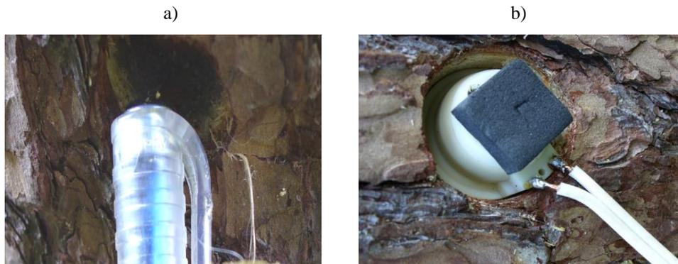
Fig. 5. Acoustic slots: a) receiving unit, b) transmitter with acoustic wave propagator
