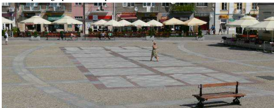
Fig. 6. Drawing of scales building foundations in the floor. Photo by the author
