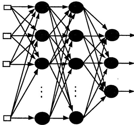
Fig. 3. A multi-layer perceptron with two hidden layers.
