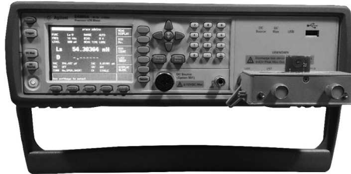
Rys. 1. Miernik RLC Keysight E4980A z adapterem 16047E Fig. 1. RLC meter Keysight E4980A with fixture 16047E.
