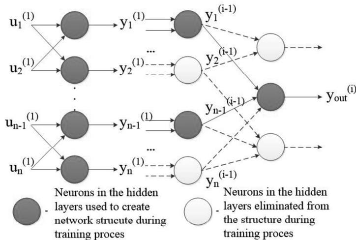
Fig. 2. A sample structure of a GMDH type neural network.
