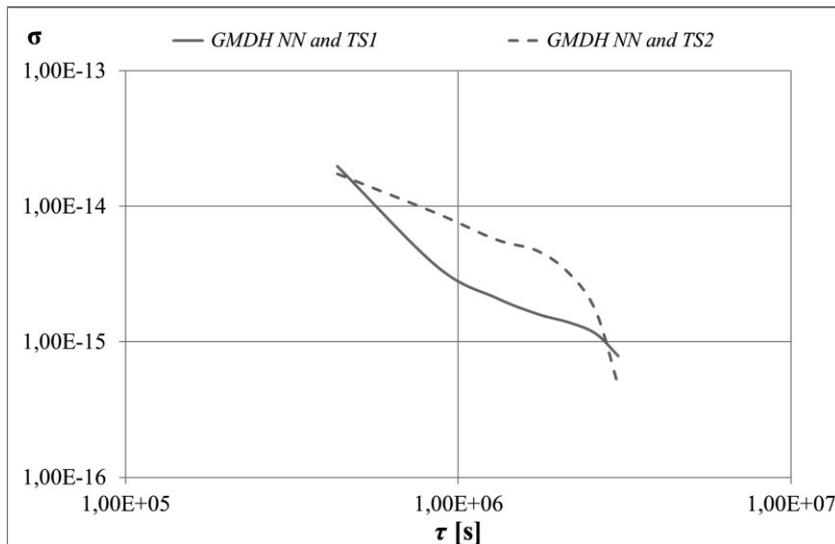
Fig. 7. The relationship MDEV of averaging time ( $\tau$ ) for GMDH neural network with time series TS1 and TS2 for UTC(PL).
