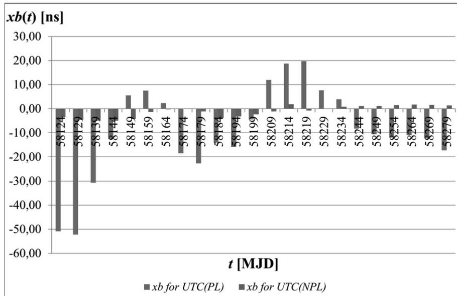
Fig. 4. Determined by the BIPM values of  $xb(t)$  deviations for UTC(PL) and UTC(NPL).
