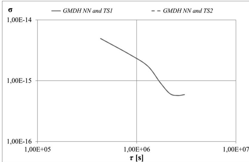
Fig. 8. The relationship MDEV of averaging time ( $\tau$ ) for GMDH neural network with time series TS1 and TS2 for UTC(NPL).
