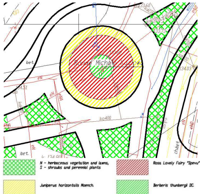
Fig. 5. Run of the hard infrastructure through the central island of Michał Kaziów roundabout, the vegetation has been marked with colour circles
