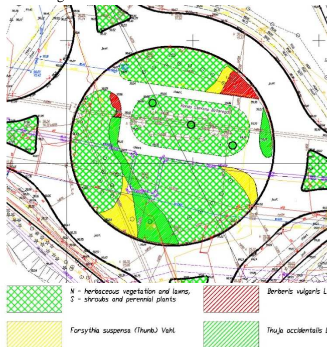
Fig. 3. Run of the hard infrastructure through the central island of Stefan Batory roundabout including plants
