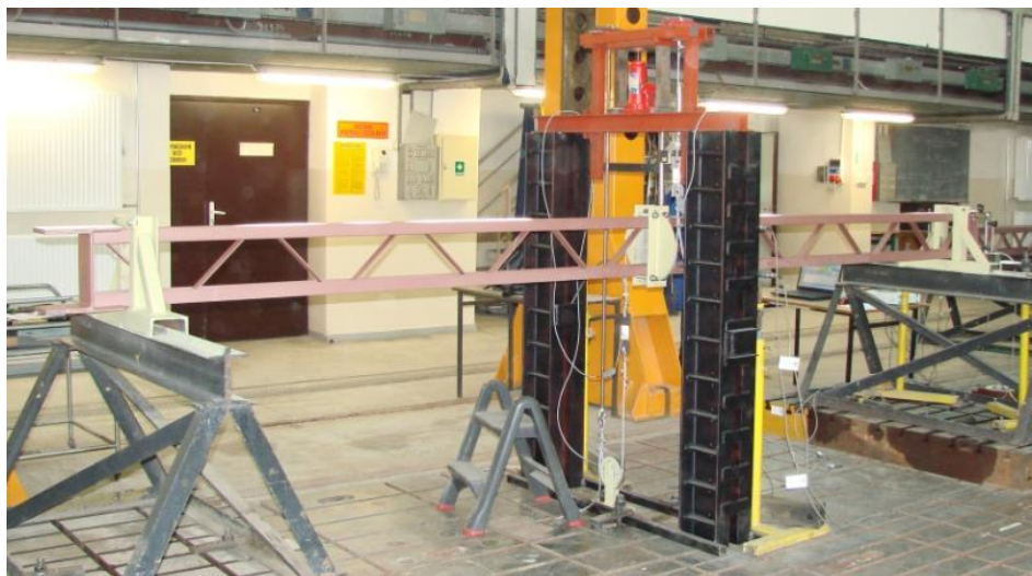
Fig. 4. Model of type S on the test stand designed for torsion
