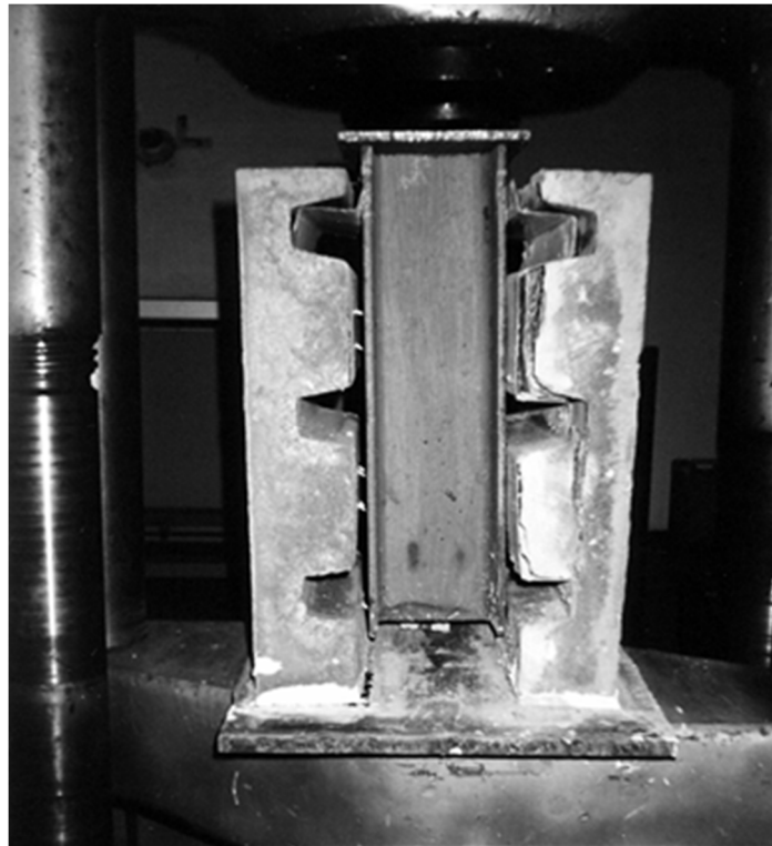
Fig. 3. Deformation form of the examined connection
