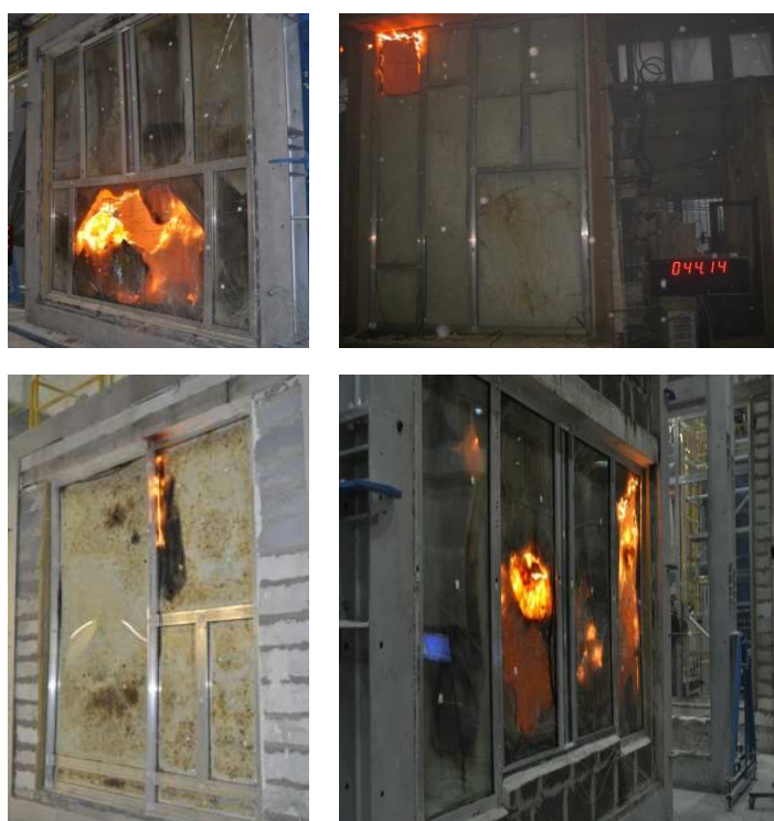
Fig. 5. Unexposed surface of tested specimens in the time of integrity failure [15]
