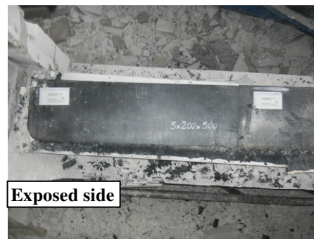
Linear joint seal No. III extent of thermal degradation – 52,7 mm
