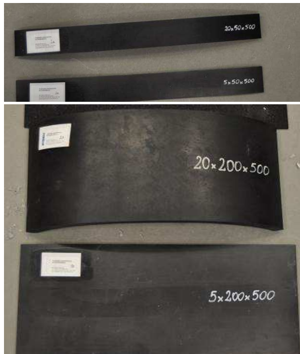
Fig. 1. Elastomer spacers used for the fire test
