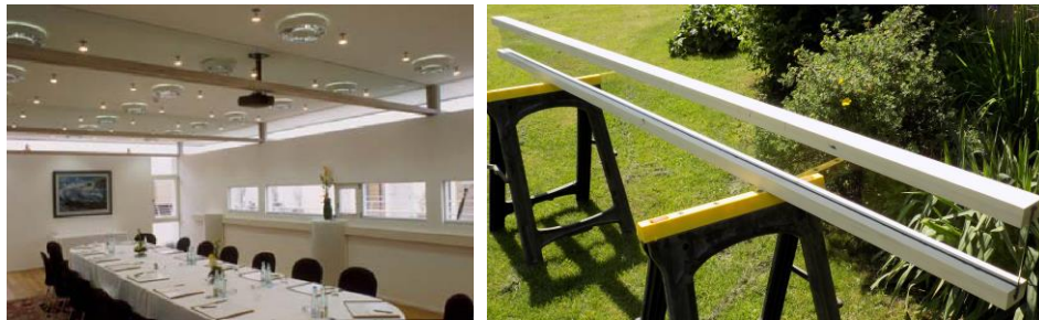
Fig. 1. Flat roof structure in the Palafitte Hotel, Switzerland [1] (left), timber-glass beam prepared for own test (right)
