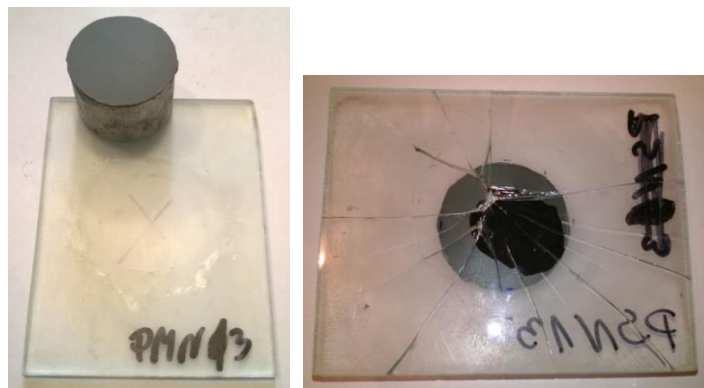
Fig. 8. Failure in glass-adhesive zone (left) and glass failure on bending (right)
