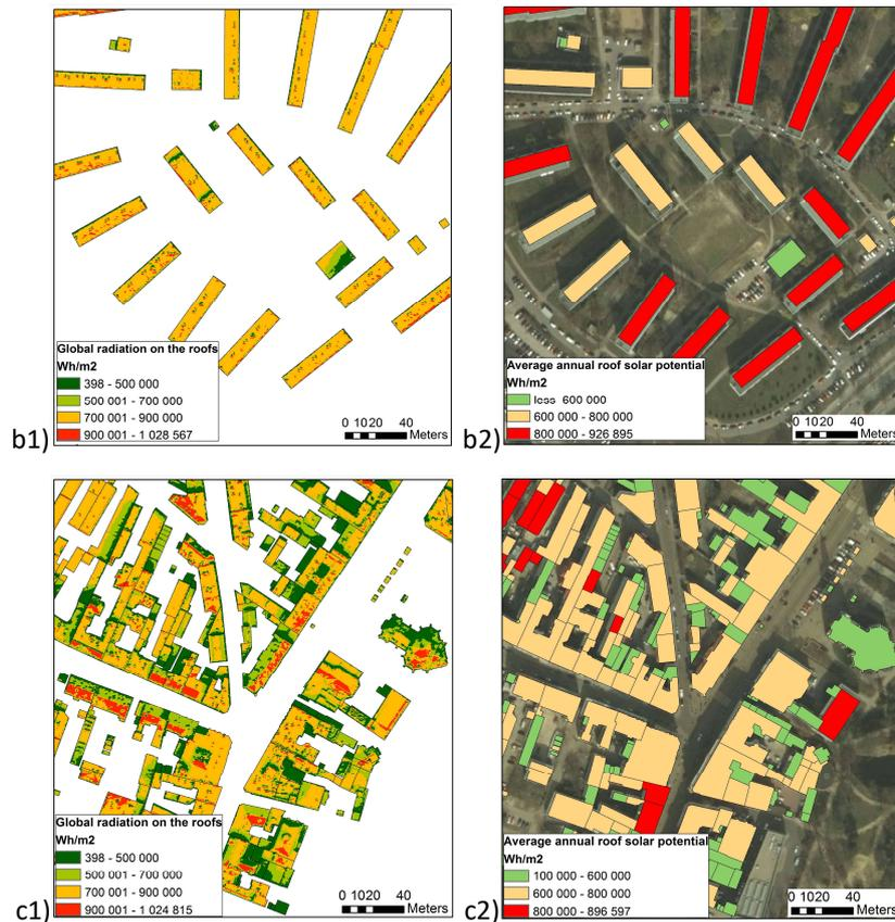
Fig. 6. Global radiation on building roofs (1) and solar potential of roofs (2) in Wh/m<sup>2</sup> in Bydgoszcz: a) a single-family housing estate; b) multi-family housing estate; c) city centre
