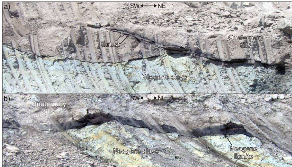
Fig. 7. Glaciotectionic deformations in the Józwin IIB opencast, Konin Lignite Mine in central Poland: a) thrust, b) inversion of the Neogene clays and lignites
