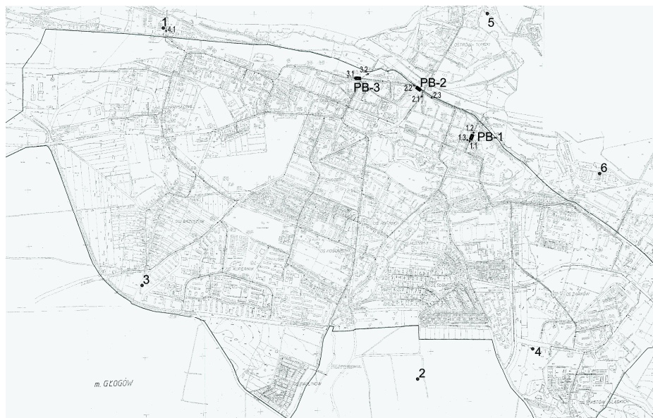
Fig. 1. Location of rain gauges and measurement stations in the area of the city in the period 2011-2014: PB-1-4 - overflow structures; 1.1-4.1 - measurement stations; 1-6 - rain gauges [3]
