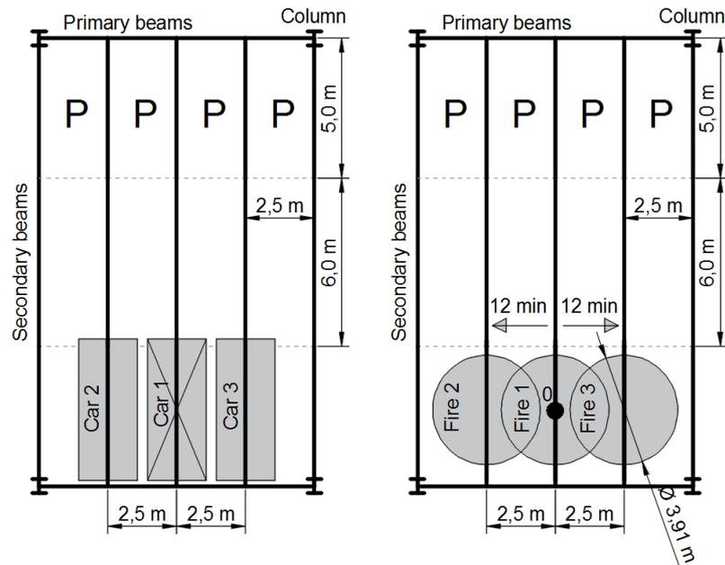
Fig. 1. Fire scenario – three cars in a line
