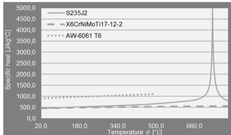
Fig. 5. Specific heat for the analysed metals
