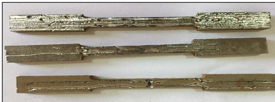
Fig.5B. Tensile sample after ultrasonic peening.
