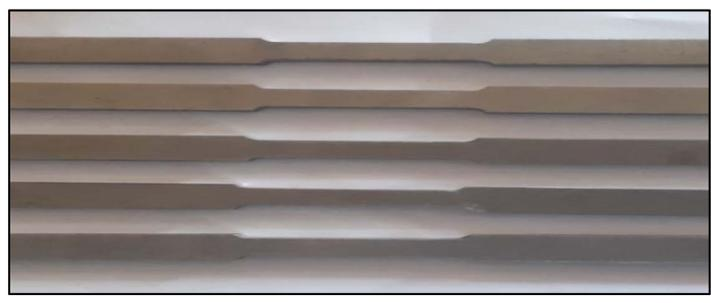
Fig.3B. Tensile specimens before ultrasonic peening process.
