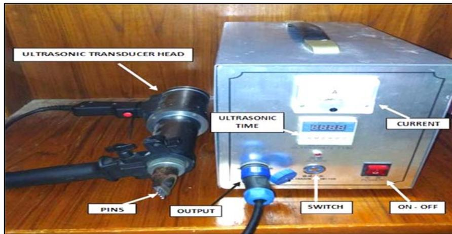
Fig.5A. The ultrasonic peening device.
