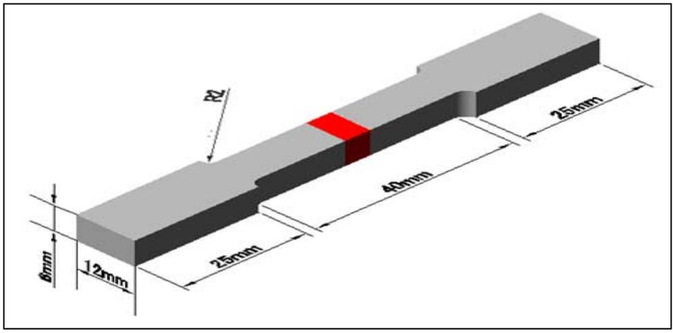
Fig.3A. Tensile sample dimensions.
