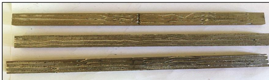
Fig.5C. Bending specimen after ultrasonic peening process
