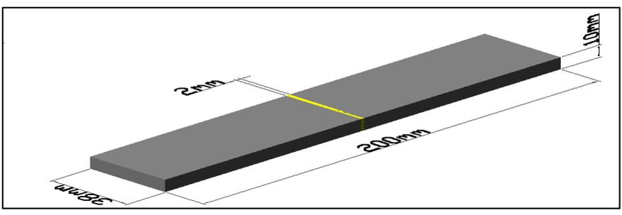
Fig.4A. Dimensions of bending specimen.
