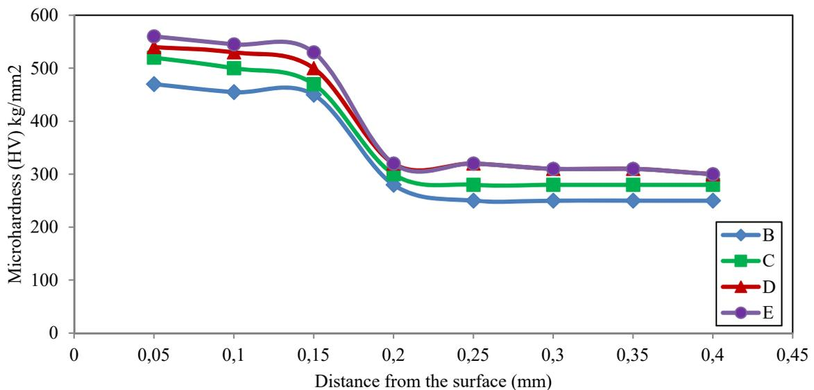
Fig.6. Micro-hardness distribution for all specimens.
