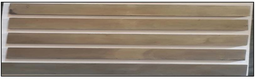
Fig.4B. Bending specimen before ultrasonic peening process.
