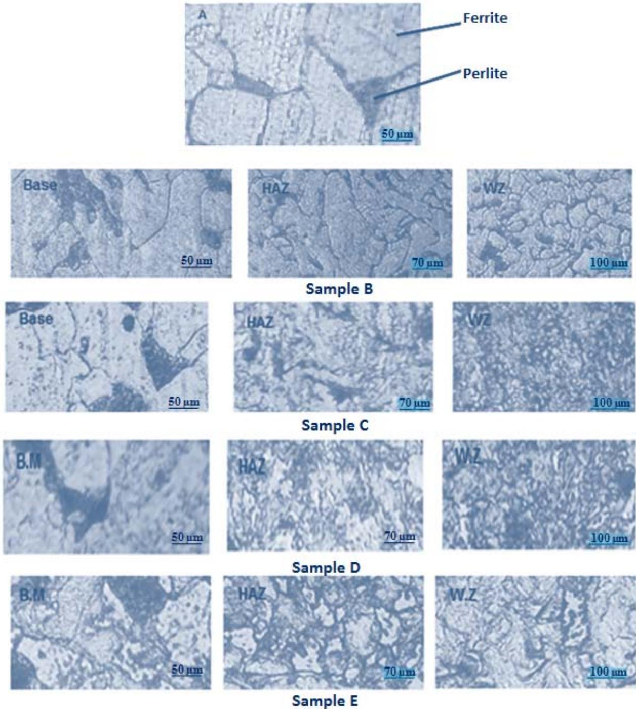
Fig.7. Microstructure of the base metal and peened and unpeened weld joints.
