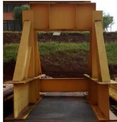
Fig.12. Gantry to be used in compression testing.
