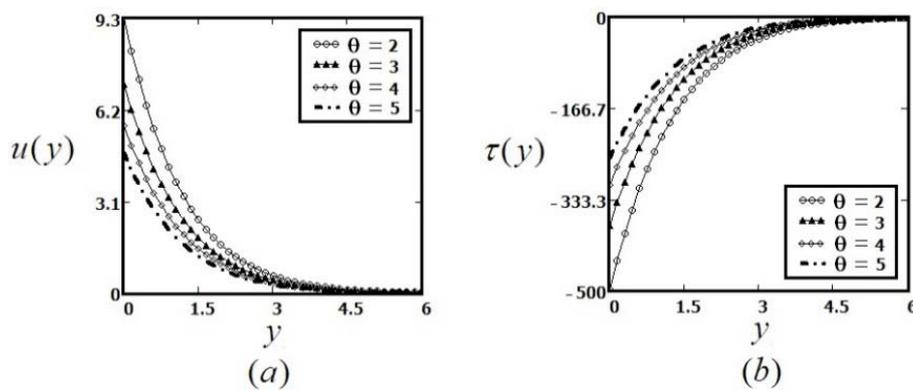
Fig.6. The velocity and shear stress profiles for  $U=1$ ,  $\nu=0.295$ ,  $\mu=26$ ,  $\alpha=0.5$ ,  $\beta=0.2$ ,  $n=2$ ,  $t=5s$  and different values of  $\theta$ .
