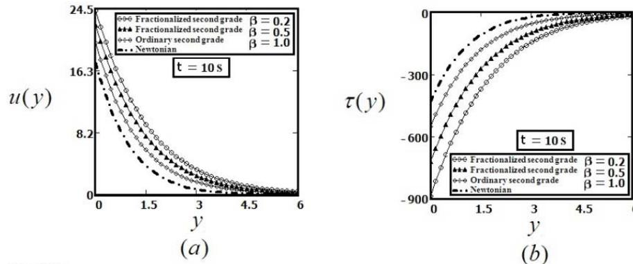
Fig.10. The velocity and shear stress profiles for  $U = 1$ ,  $\nu = 0.295$ ,  $\mu = 26$ ,  $\alpha = 0.5$ ,  $\beta = 0.2, 0.5, 1$ ,  $\theta = 5$  and  $t = 10s$ .
