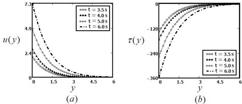
Fig.2. The velocity and shear stress profiles for  $U = 1, \nu = 0.295, \mu = 26, \alpha = 0.5, \beta = 0.2, \theta = 5, n = 2$  and different values of  $t$ .
