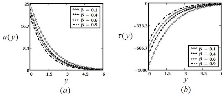
Fig.5. The velocity and shear stress profiles for  $U=1$ ,  $\nu=0.295$ ,  $\mu=26$ ,  $\alpha=0.5$ ,  $\theta=5$ ,  $n=2$ ,  $t=4s$  and different values of  $\beta$ .
