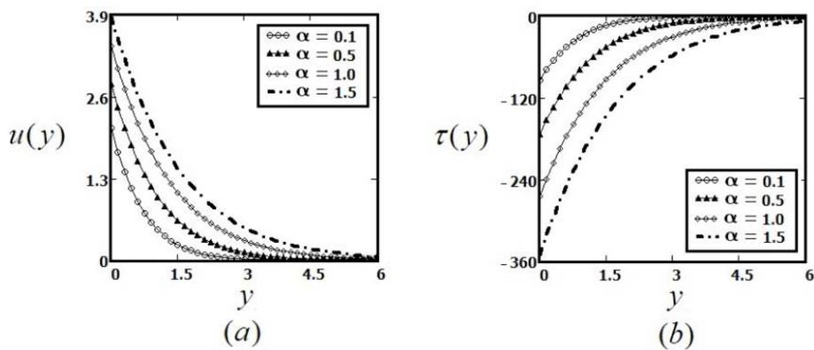
Fig.3. The velocity and shear stress profiles for  $U = 1, \nu = 0.295, \mu = 26, \beta = 0.2, \theta = 5, n = 2, t = 4s$  and different values of  $\alpha$ .
