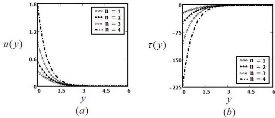
Fig.7. The velocity and shear stress profiles for  $U = 1$ ,  $\nu = 0.295$ ,  $\mu = 26$ ,  $\alpha = 0.5$ ,  $\beta = 0.2$ ,  $t = 2s$  and different values of  $n$ .
