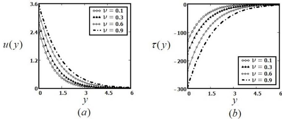
Fig.4. The velocity and shear stress profiles for  $U=1$ ,  $\rho=88$ ,  $\alpha=0.5$ ,  $\beta=0.2$ ,  $\theta=5$ ,  $n=2$ ,  $t=4s$  and different values of  $\nu$ .
