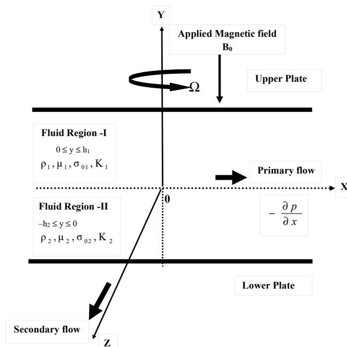
Fig.1. Schematic flow diagram.
