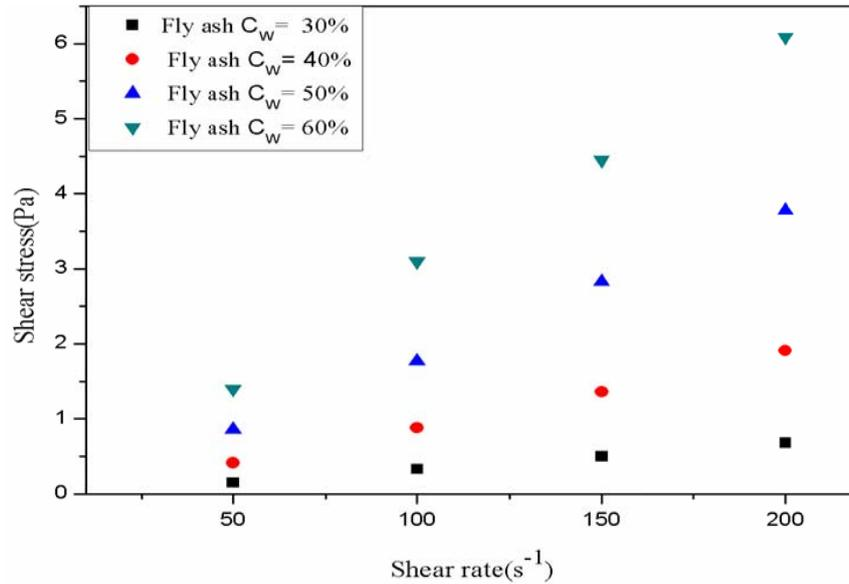
Fig.5. Shear stress-shear rate curve of fly ash.
