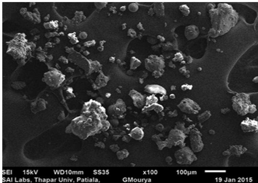
Fig.1. SEM of fly ash sample.
