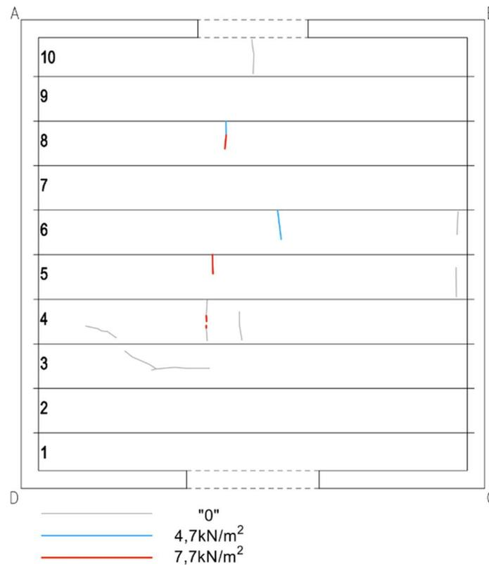
Fig. 15. Crack patterns on the bottom surface
