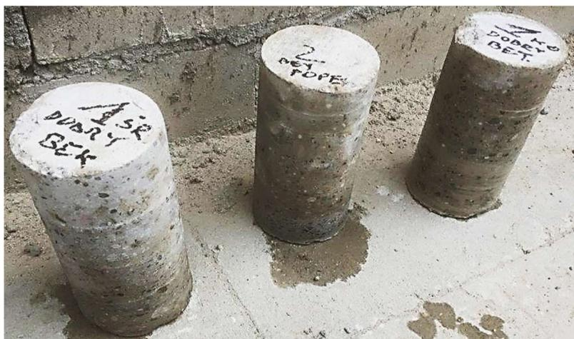
Fig. 19. Cores from the mid-span and support zones
