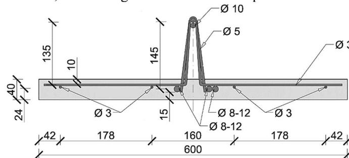
Fig. 1. Vector II cross-section [1]
