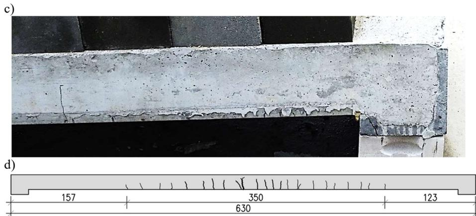
Fig.17. Cracks of the strip model: a) load  $17.3 \text{ kN/m}^2$ , b) crack in the middle of the span after failure, c) cracks near the support, d) view of cracks along the length of the slab after failure
