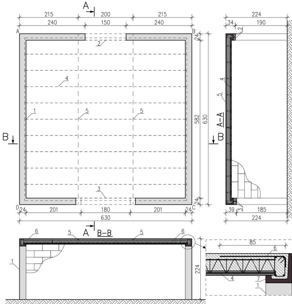
Fig. 4. Geometric dimensions: top view, A-A cross-section, B-B cross-section (1-wall, 2-lintel  $2 \times$  SBN 7,2/12/210, 3- lintel  $2 \times$  SBN 12/12/180, 4- Lattice girder panel, 5- distribution ribs, 6- support reinforcement, 7- precast form)
