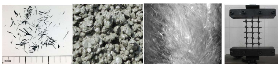
CCFCM- Fibers steel fibers in PC Mix waste plastic fiber geogrid
