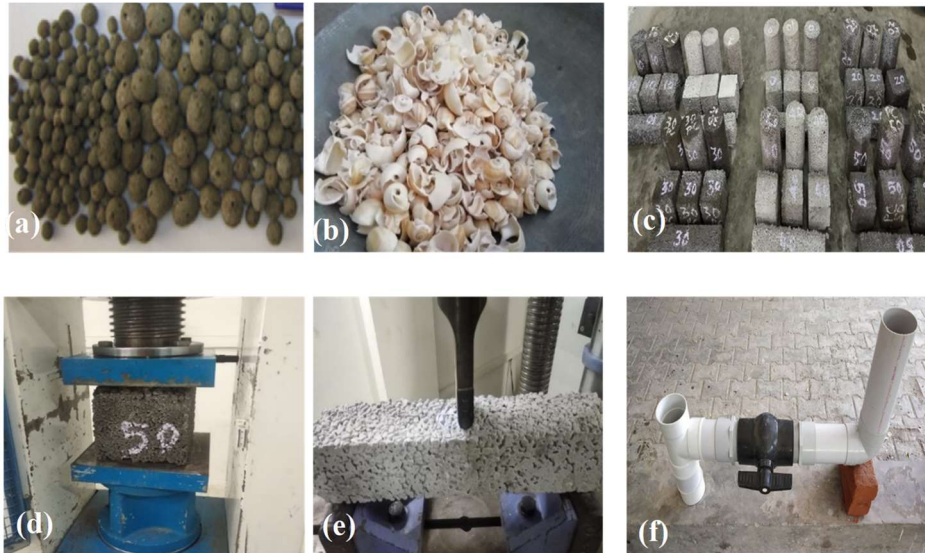
(a) Expanded Clay aggregate; (b) Crushed Seashell; (c) Casted specimen; (d) Compression test (e) Split tensile Strength test (f) Falling head Permeability test
