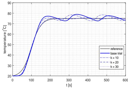
Figure 10: Time responses, PID controller
