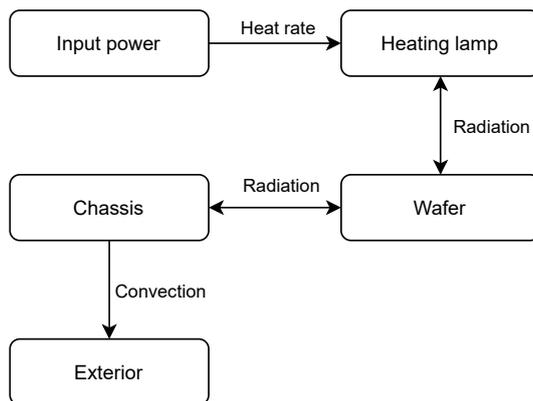
Figure 2: Energy transfer diagram
