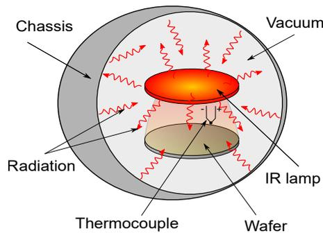
Figure 1: Scheme of vacuum furnace
