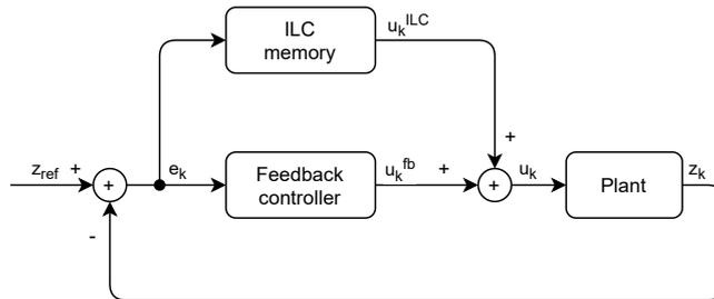
Figure 3: Feedforward ILC scheme
