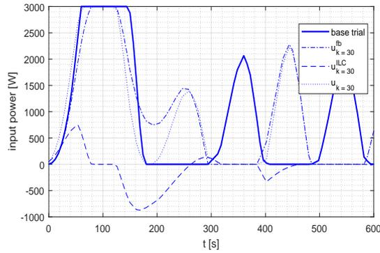
Figure 9: Input signal composition, PI controller
