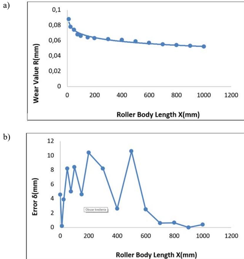
Fig.2. Comparison of measured and model predicted value of work roll 1 (a: Measured and predicted value of work roll 1, b: Relative error of measured and predicted value of work roll 1).
