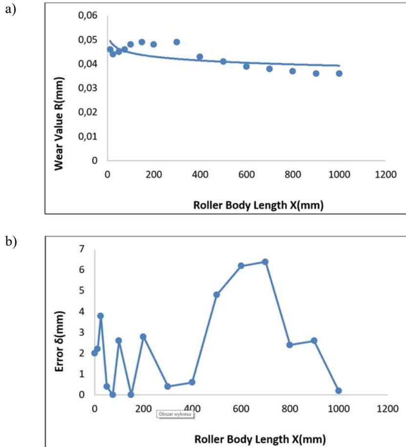
Fig.3. Comparison of measured and model predicted value of work roll 2 (a: Measured and predicted value of work roll 2, b: Relative error of measured and predicted value of work roll 2).
