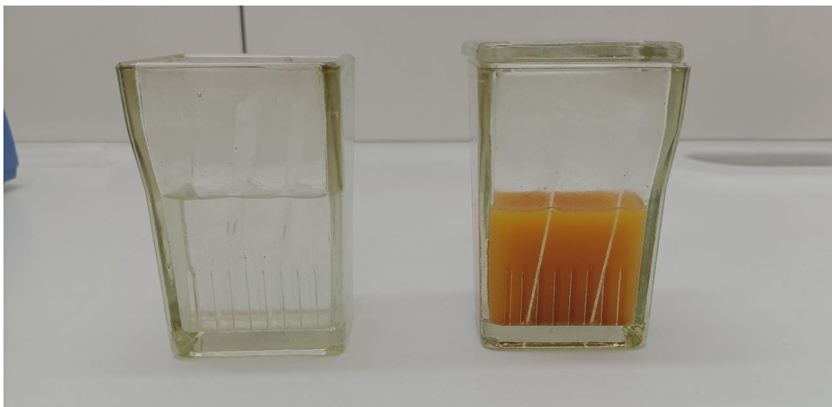
Fig. 3. Laboratory set-up for the slide stain experiment. On the left 30% \text{H}_2\text{O}_2 , on the right Fenton's solution. Two slides each with samples applied in both containers
