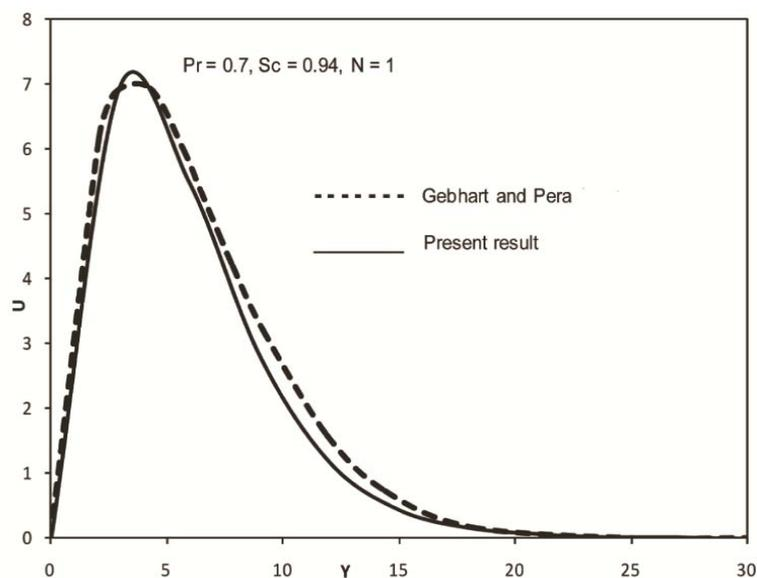
Fig.3. Velocity profiles comparison with Gebhart and Pera [1].
