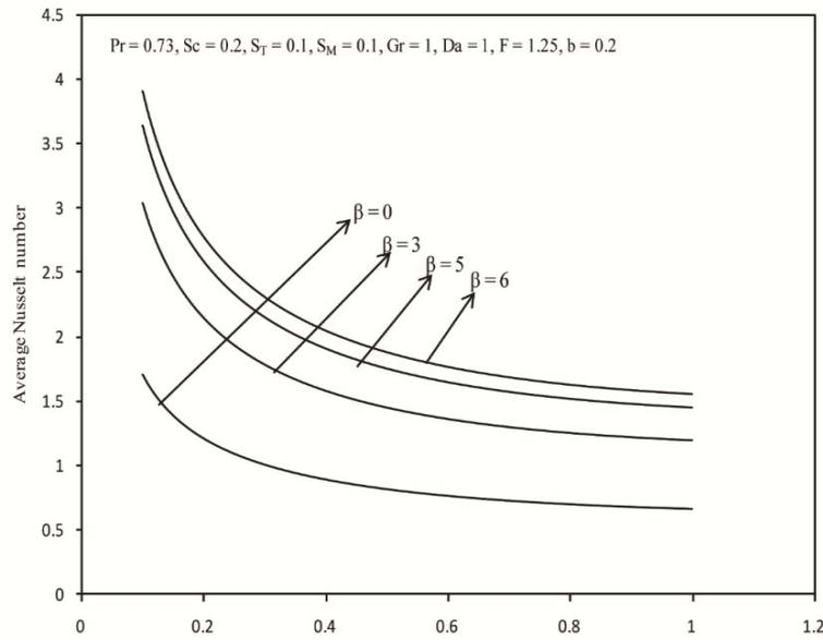
Fig.18. Effect of varying thermal conductivities on average Nusselt number.
