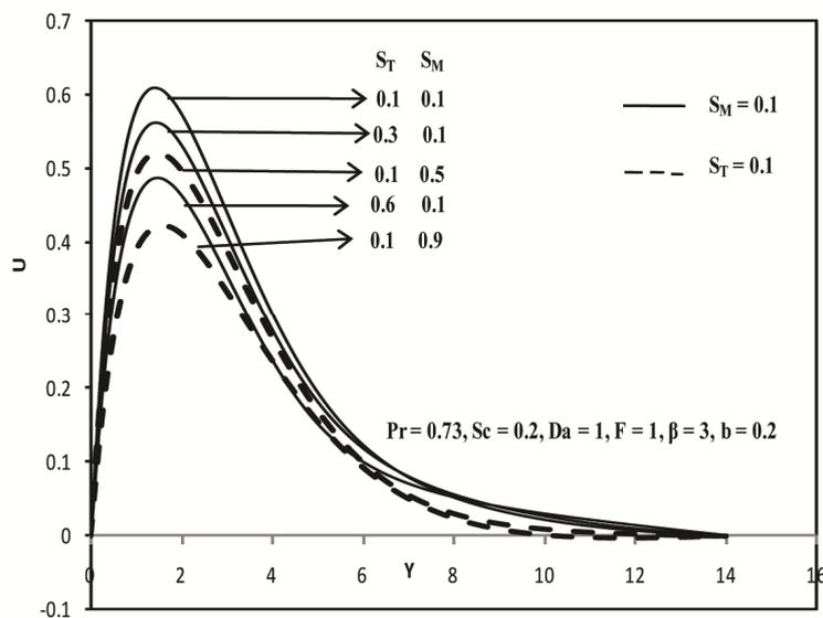
Fig.5. Influence of  $S_T$  and  $S_M$  on velocity profiles.
