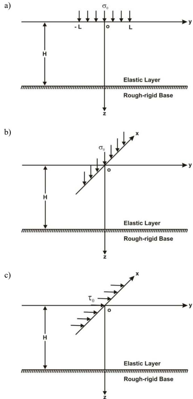
Fig.1. A uniform, elastically isotropic layer of finite thickness  $H$  overlying a rough-rigid base being acted upon by (a) normal strip loading  $\sigma_0$  in the positive  $z$ -direction uniformly distributed over the strip  $-L \leq y \leq L$  (b) normal line loading  $\sigma_0$  per unit length in the positive  $z$ -direction (c) shear line loading  $\tau_0$  per unit length in the positive  $y$ -direction.
