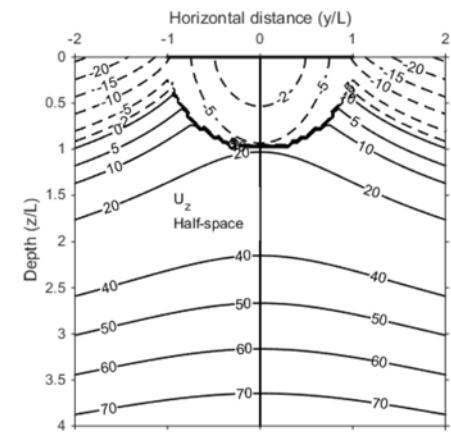
Fig.6. Contour map of the normalized vertical displacement  $U_z$  for normal strip loading  $-L \leq y \leq L, z = 0$  for (a) layer thickness  $H = 2L$  (b) Half-space.
