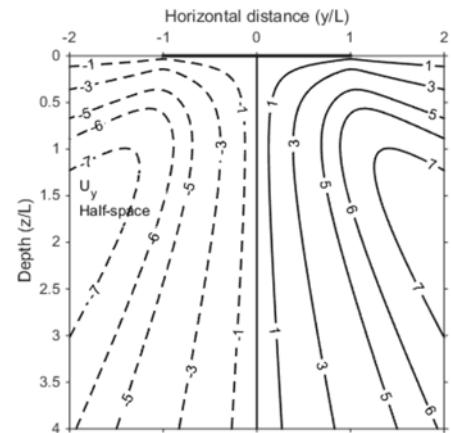
Fig.5. Contour map of the normalized horizontal displacement  $U_y$  for normal strip loading  $-L \leq y \leq L, z = 0$  for (a) layer thickness  $H = 2L$ , (b) half-space.
