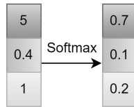
Fig. 5. Illustration of the softmax operation.
